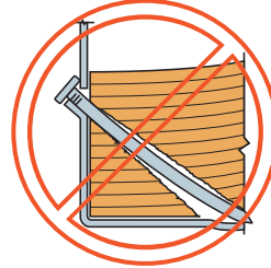
Nail Too Long
